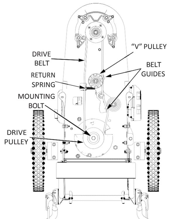
FIGURE 15: Routing The Drive Belt
