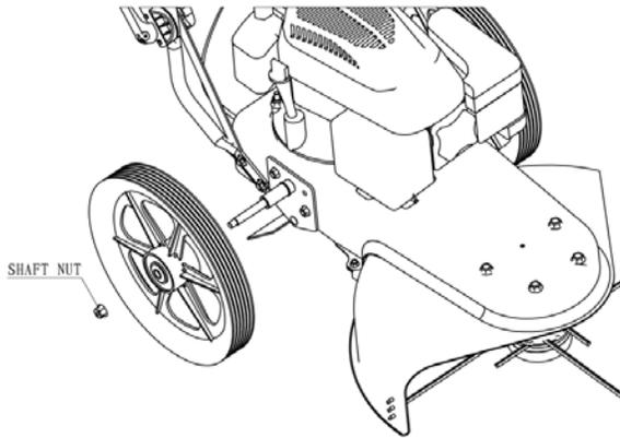
**FIGURE 11:** Removing the Wheels.
