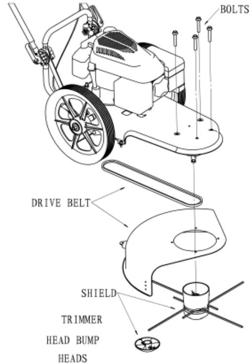
FIGURE 14: Mower Head Housing and Shield
